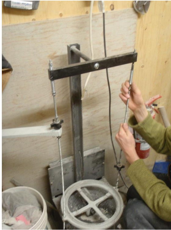
Photo 5: Repairing the sieve shaker in the geotechnical lab.
